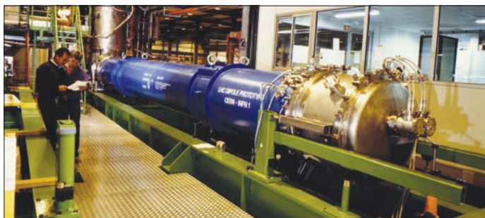
Fig. 7. On 14 April 1994 the first 10 m LHC dipole prototype from INFN was successfully powered at CERN for the first time. This magnet is now operating in the CAST experiment at CERN.
