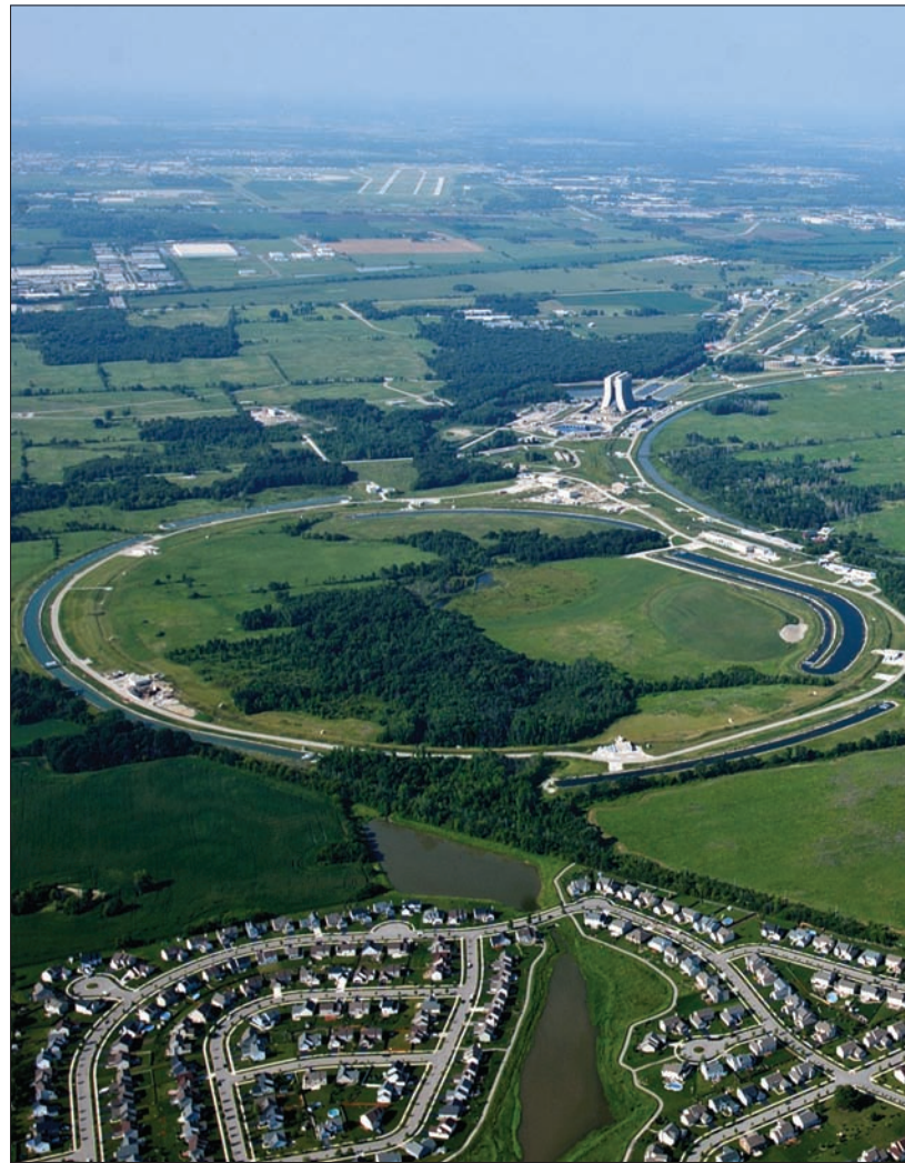
The Fermilab site. The Tevatron is the large ring to the right and the Main Ring to the left.
