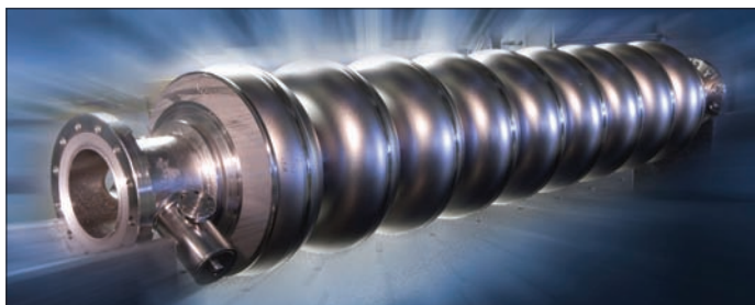
XFEL cavities reach 30–40 MV/m and will be used for the ILC. (Image credit: Fermilab Visual Media Services.)
