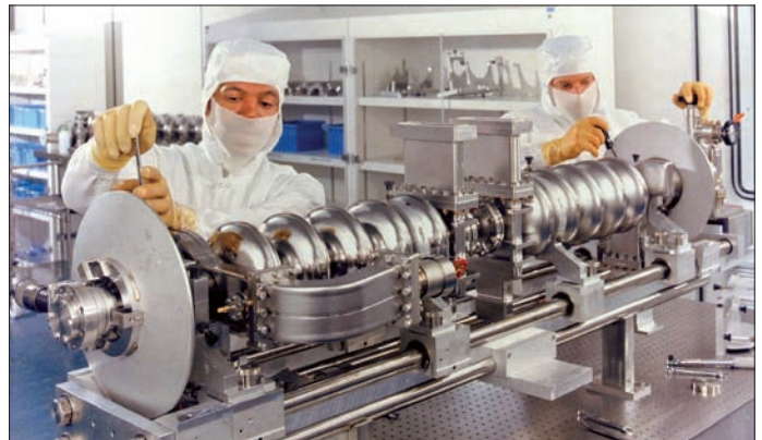
Cornell/Jefferson Lab cavities run CEBAF at 7–10 MV/m. (Image credit: Jefferson Lab.)
