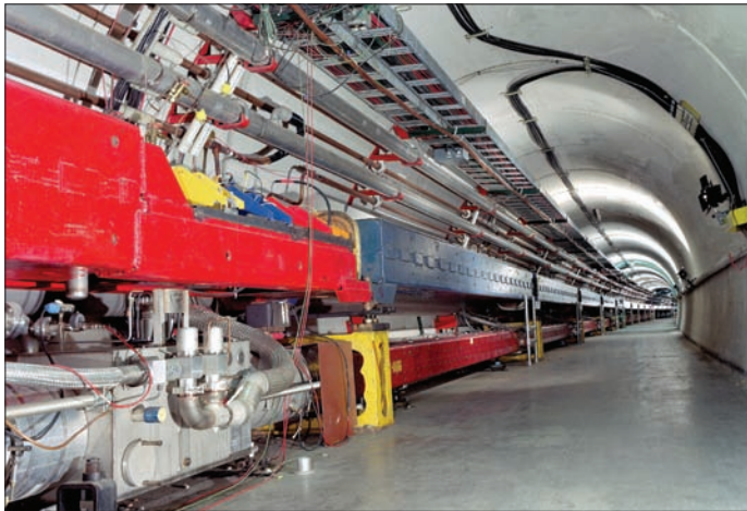
The Tevatron ring with red dipoles fit neatly beneath the original Main Ring with its blue dipoles, as Robert Wilson had foreseen. (Image credit: Fermilab Visual Media Services.)
