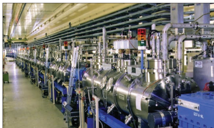
Fig. 4. The superconducting cavity string used for beam acceleration in TRISTAN.
